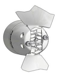
**8** Tighten both pivot pin locking screws (9) using the Allen wrench (15) supplied; If using torque wrench tighten to about 1.2 Kpm=12 Nm=8.4 ft-lb;
