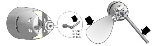
2 Slide tab washer (5) on to shaft nut locking screw (6); screw in through hole in the shaft nut into end of shaft and tighten firmly; If using torque wrench tighten to about 0,5 Kpm=5 Nm=3,6 ft-lb;
