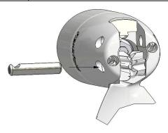
**5** Insert one pivot pin locking screw (9); turn it to engage a couple of threads; It will be tightened later in step 8;
