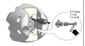
**3** Again using a straight screw driver: Bend side of tab washer up over hex on the shaft nut locking screw (6).
