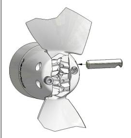
7 Insert last pivot pin locking screw (9); turn it to engage a couple of threads; It will be tightened later in step 8;
