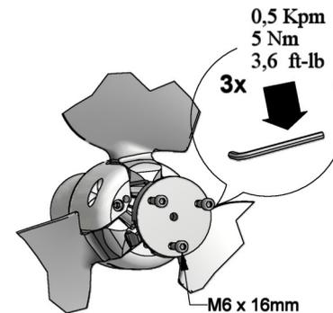
**6** Mount sacrificial anode (11) Zn or AlMg, with one socket-head cap screw (12) after having applied thread locker to threads if not already applied.
