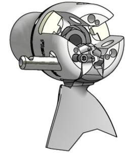
**4** Continue with the next two blades; Work blades open and folded to ensure ease of operation; Tighten all pivot pin locking screws using the Allen wrench supplied. If using torque wrench tighten to about 1.2 Kpm = 12 Nm = 8.4 ft-lb.; Again work blades open and folded to ensure ease of operation;
