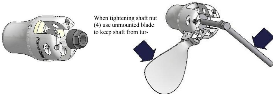
**2** Mount shaft nut locking screw (5) using the Allen wrench (13) supplied. If using torque wrench tighten to about 1 Kpm=10 Nm=7.2 ft-lb;
