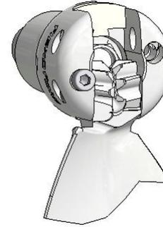
**5** Align last blade (6) in hub jaw and insert pivot pin (7) with the notch in pin aligned with the hole for the pivot pin locking screw; Move blade slightly to ease operation;
