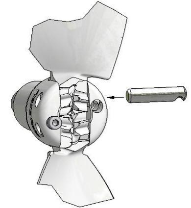
**6** Insert last pivot pin locking screw (8); turn it to engage a couple of threads; It will be tightened later in step 7;
