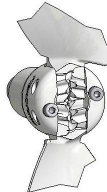
**7** Tighten both pivot pin locking screws (8) using the Allen wrench (10) supplied; If using torque wrench tighten to about 1.2 Kpm=12 Nm=8.4 ft-lb;
